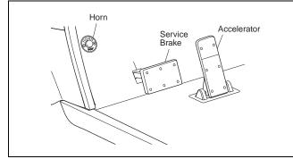
Fig. 11 Accelerator, Brake and Horn
